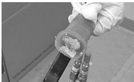
**Change nozzles frequently!** Foam will cure inside the nozzle in the same amount of time that foam becomes tack-free in the air.
