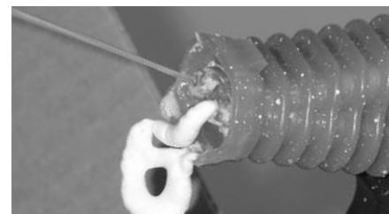
Partial or complete blockage of one chemical port will result in off-ratio foam.
