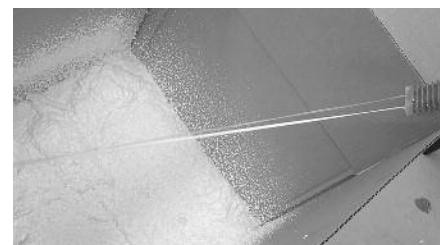
With the nozzle removed, check that both chemicals flow with equivalent force.
