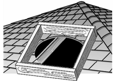
Fig. 2 - Mounting the Curb Box
